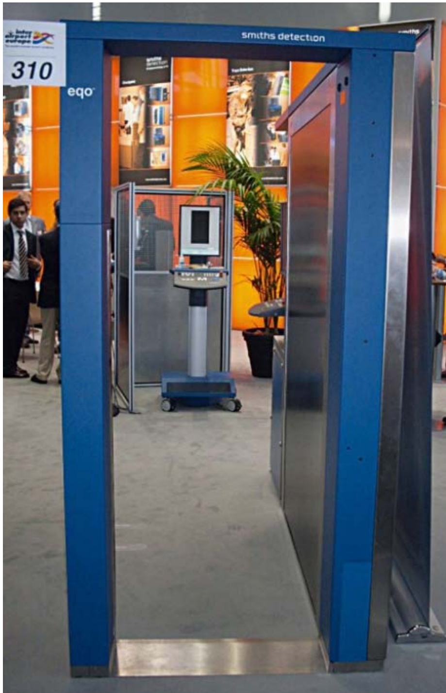
The eqo MMW full-body scanner from Smiths Detection resembles a standard walkthrough portal. (IHS Jane's/Ben Vogel) 1354586
